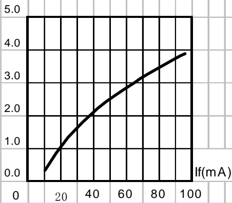
Fig.3 RELATIVE LUMINOUS INTENSITY VS. FORWARD CURRENT.
